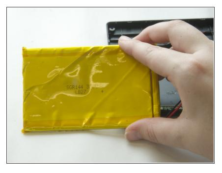
Gently remove the battery, with the wires, from the panel and motherboard completely. To reassemble your device, follow these instructions in reverse order.
