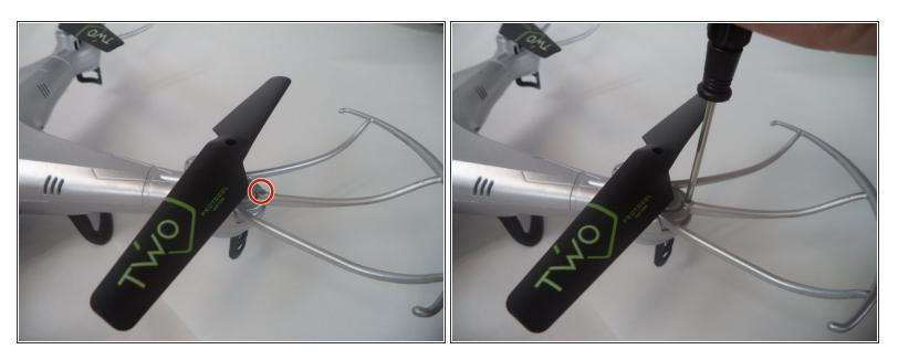
• Using your screwdriver, remove the 8.36mm Phillips screw.
