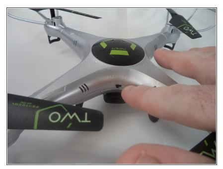
• Turn the drone off by moving the selector switch to the left.
