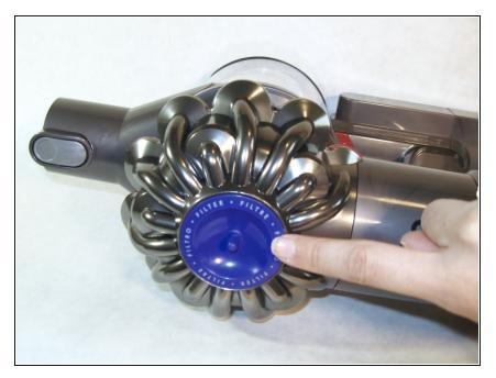
• Locate the blue knob labeled "Filter" at the center of the cyclone.
