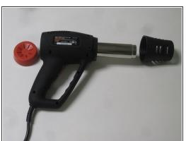
Remove the barrel casing on either end by twisting and pulling each side off.
