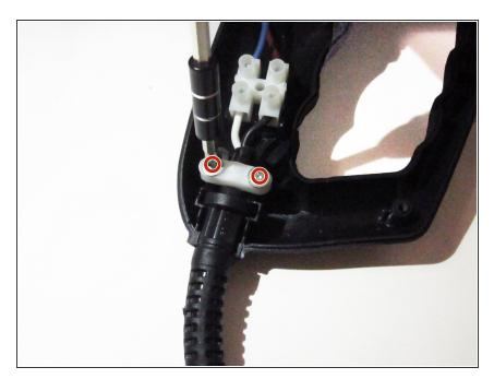
Remove the two 12mm screws from the base of power cord using the PH#0 screwdriver.
