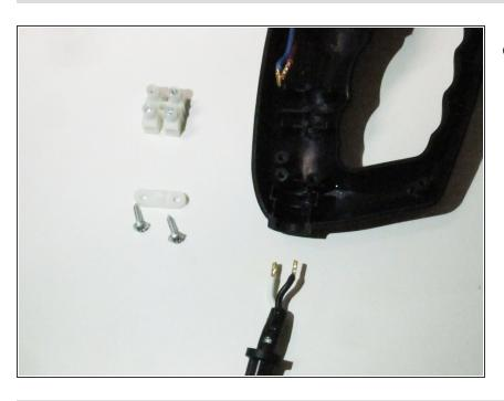
Remove the power cord from the heat gun.
