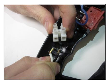
Disconnect the power cord wiring from the wire connector.
