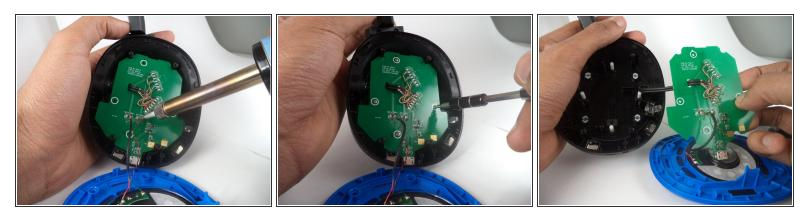
• Desolder the necessary wires. (Each side will be slightly different.)
