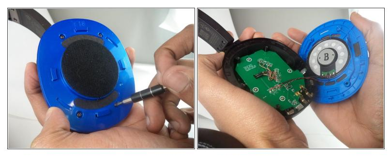
Remove the screws (9.47 mm Phillips head) from the blue plating on the headset to reveal the inside.
