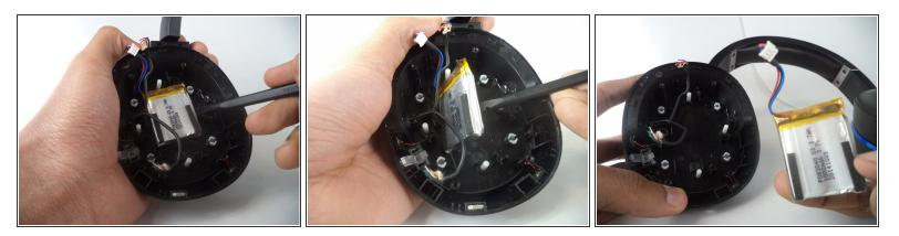
• Remove the battery by carefully prying it from the headset.
