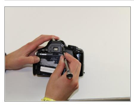
Using the PH000 screwdriver, remove the four 4mm screws behind the eyepiece.
