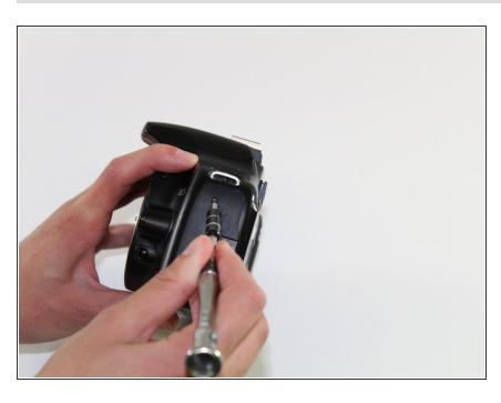
Using the PH000 screwdriver head, remove one 4 mm screw on the left side of the camera (from the LCD screen).
