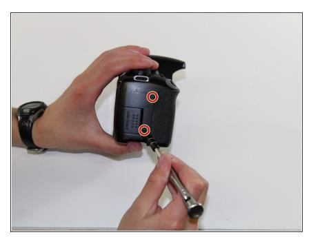
Using the PH000 screwdriver head, remove the two 3mm screws on the right side of the camera (from the LCD screen).
