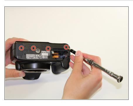
Using the PH000 screwdriver head, remove the four 4 mm screws on the bottom of the camera.
