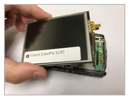
Lift the LCD screen away from the camera. To reassemble your device, follow these instructions in reverse order.
