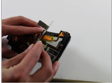
Remove the metal plate covering inside of the LCD screen
