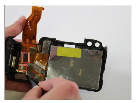
Carefully disconnect the circuitry sheets from the white plastic bases
