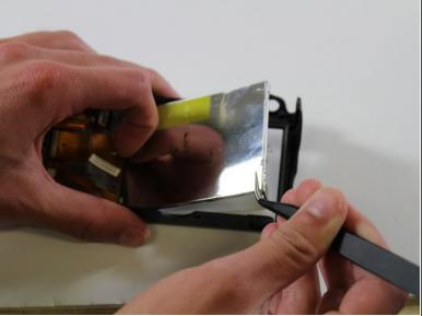
Using the plastic spudger, carefully pry out the LCD screen from the back panel
