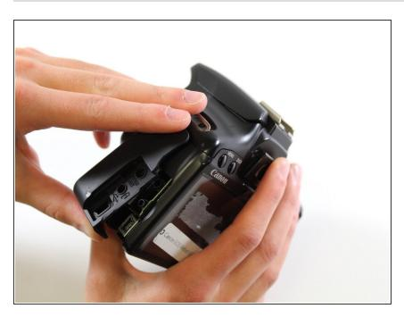
Remove the side panel by lifting off with fingers.
