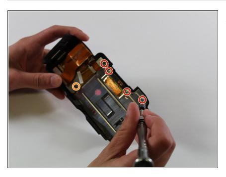
Using the PH00 screwdriver head, unscrew four 4 mm screws and one 2 mm screw
