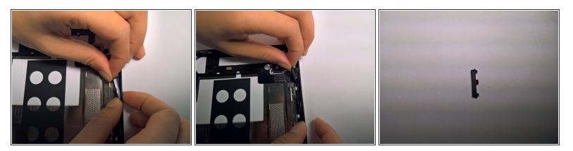
• From the outside edge of the device, carefully push the volume button inwards towards the middle of the device.
