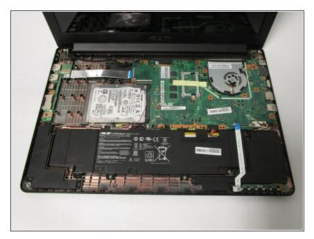
Remove the keyboard panel completely and set it aside. The internal components of the laptop are now exposed.
