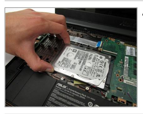
Slide the hard drive in the direction away from the connector and lift it up to remove it.
