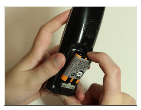
• Pull out to remove the battery.
