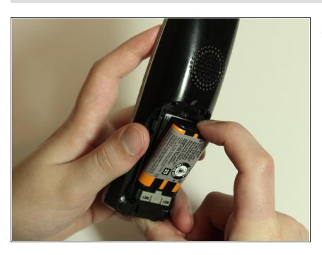
Pull out to remove the battery.
