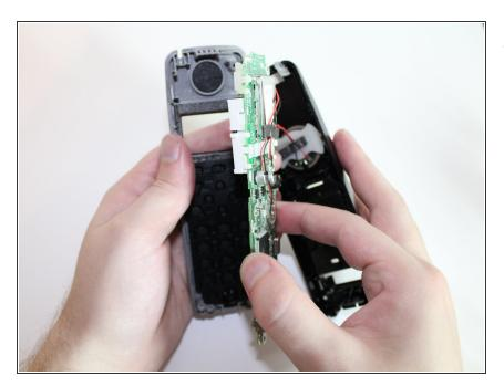
Remove the circuit board.
