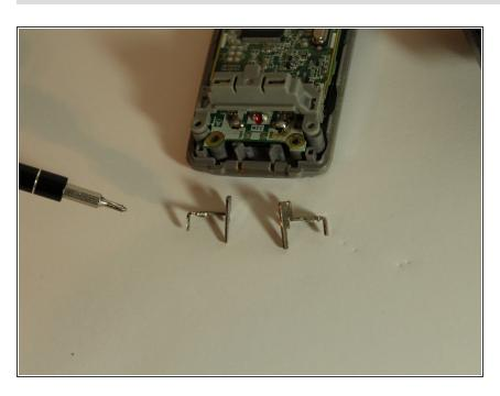
Once the screws are out, remove the charging contacts beneath the two bottom corner screws.
