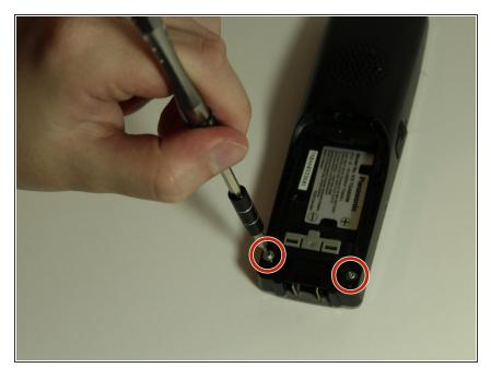
Once battery is removed, use the Phillips #00 screwdriver to remove the two silver screws at the bottom left and right corners on the back of the phone.
