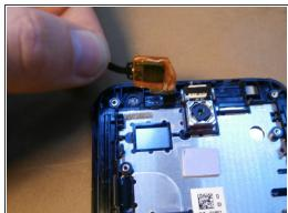
Disconnect the touchscreen driver to remove the screen
