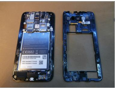
Remove the plastic back with opening picks making sure not to break the clips that hold it in place
