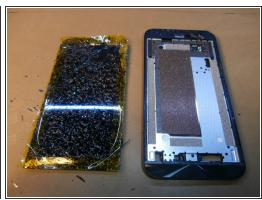
With the help of a hair dryer, heat gun or an iOpener remove the screen from the phone's frame
