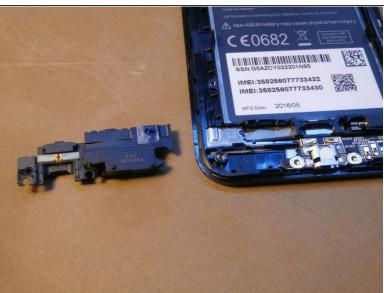
With the help from a spudger, remove the rear speaker
