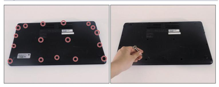
• Remove the 18 Phillips screws using a screwdriver with a PH0 bit.
