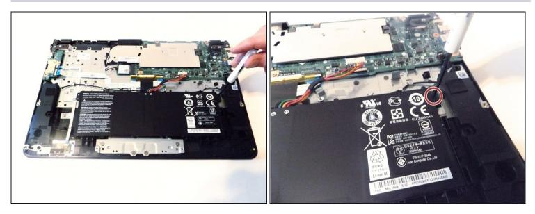
• Next, unscrew the battery pack. The one screw should be located on the far right of it. This will ensure that the battery comes out easily and affectively.
