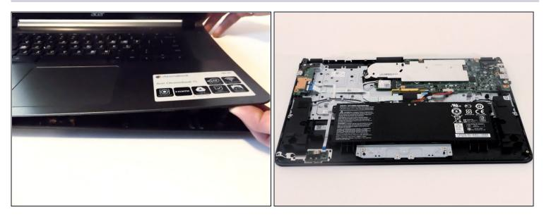
• Using a spudger, gently pry open the back from the top.
