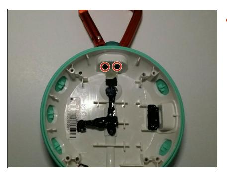
There are two 3 mm T8 screws holding the carabineer in place, remove these two screws.
