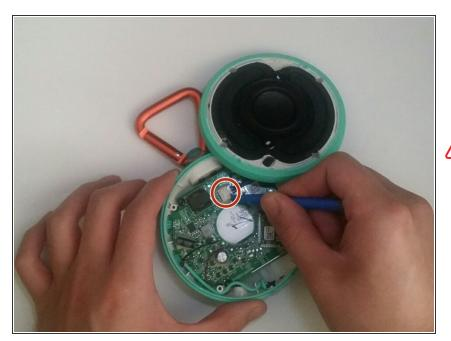
To completely remove the top portion, disconnect the speaker from the motherboard using the blue plastic opening tool.
