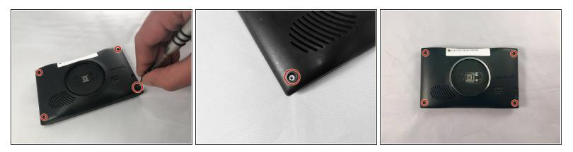
Remove the four screws on the back of the GPS using the T5 Torx screwdriver.
