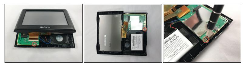
• Using the T5 Torx screwdriver, remove the two screws located on the motherboard.
