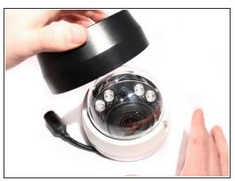
Lift off the paintable snap-on cover from the AvertX HD810 dome security camera.
