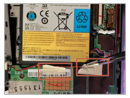
• Use tweezers to remove the tape covering the battery's wiring.
