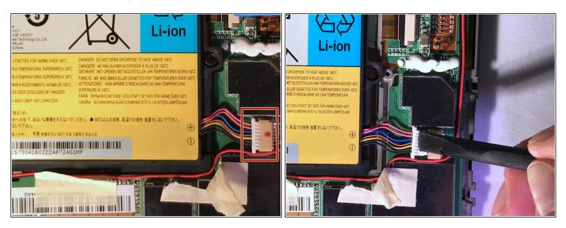
1 Do not puncture the lithium-ion battery. Ruptured batteries can catch fire or explode.
