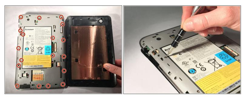
Use a Phillips #000 screwdriver to remove the seventeen 4mm screws.
