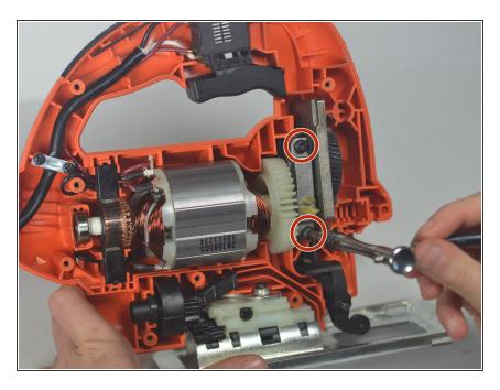
Remove the two 30.1625mm screws with a T20 torx screwdriver that are holding the gearbox to the housing.
