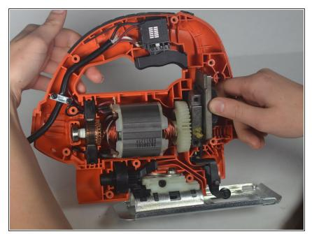
Apply a light force to separate the gearbox from the housing. This will momentarily separate the gearbox and help with the removal of the system in later steps.
