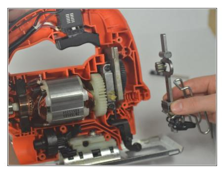
Being careful to keep all parts together, grab the entire assembly and pull it directly out of the saw.
