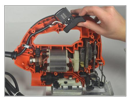
By separating the two housing halves, carefully remove the top plate.
