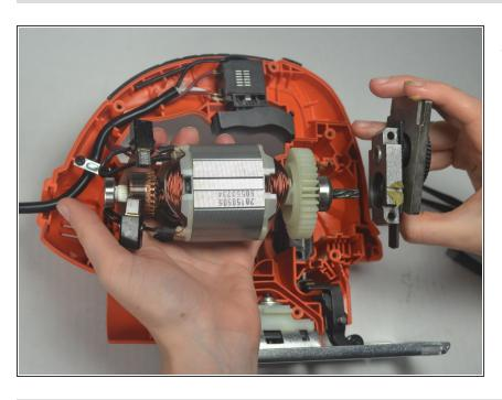
While holding the motor in one hand, gently pull the gearbox off of the drive shaft.
