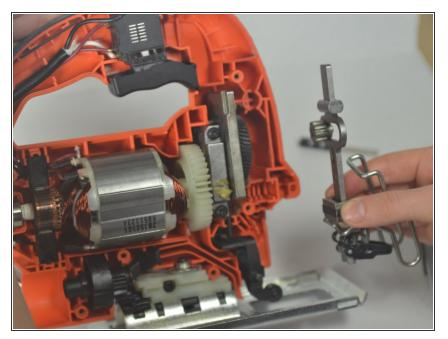
Being careful to keep all parts together, grab the entire assembly and pull it directly out of the saw.
