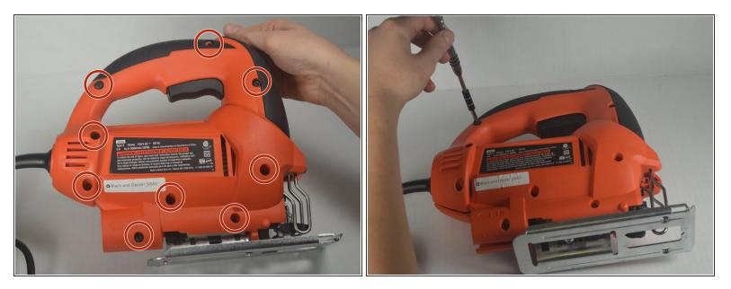
• Remove the nine torx 15.875mm screws on the front of the jigsaw using a T-15 torx screwdriver.
