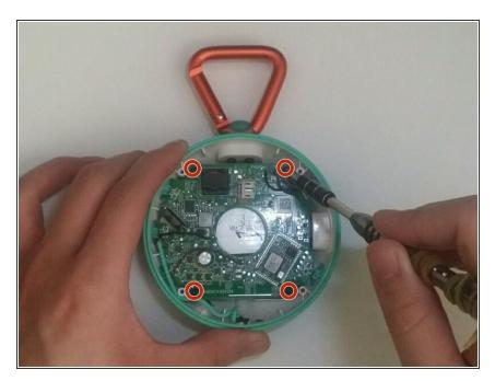
There will be four 3 mm T8 screws holding the motherboard in place, remove these four screws.
