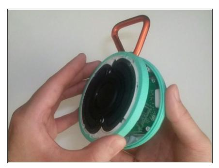
The front cover will lift open easily and the components will be visible.
