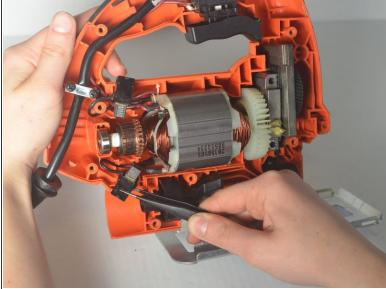
Using tweezers or a small flathead screwdriver, gently remove each of the black magnetic clasps away from the motor.
