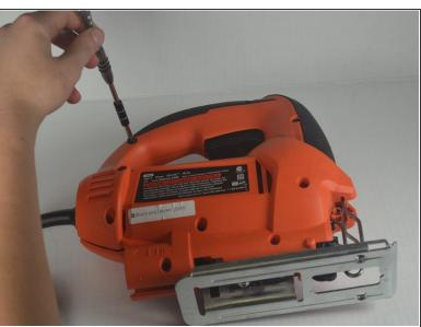
• Remove the nine torx 15.875mm screws on the front of the jigsaw using a T-15 torx screwdriver.
