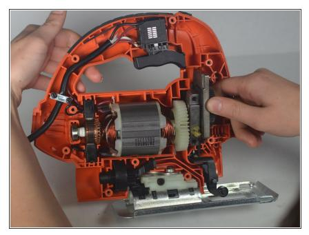
Apply a light force to separate the gearbox from the housing. This will momentarily separate the gearbox and help with the removal of the system in later steps.
