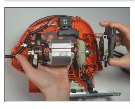
While holding the motor in one hand, gently pull the gearbox off of the drive shaft.
