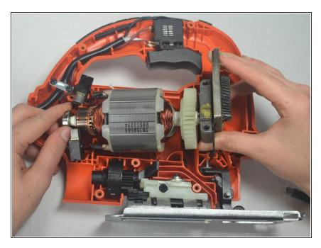
Holding the gearbox and the bering, pull the whole motor and gearbox out of the housing.
