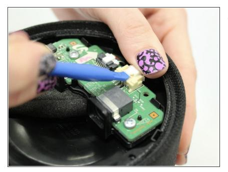
• While stabilizing the Port Panel remove the two ribbon cables one at a time by pressing the locking clip down on the ribbon cable connectors and pulling the connector away from the Port Panel.
