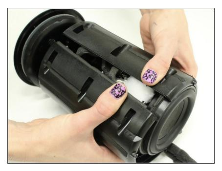
• Open up the body to expose the inner panel and motherboard.
