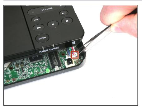
Gently remove the wires with tweezers by pulling up on the base they are attached to.
