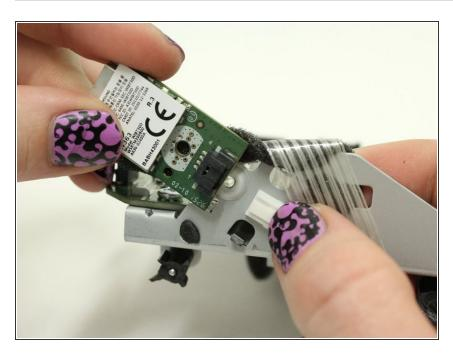
Press the white tab while gently pulling the Bluetooth module away from the connector and frame. To reassemble your device, follow these instructions in reverse order.
