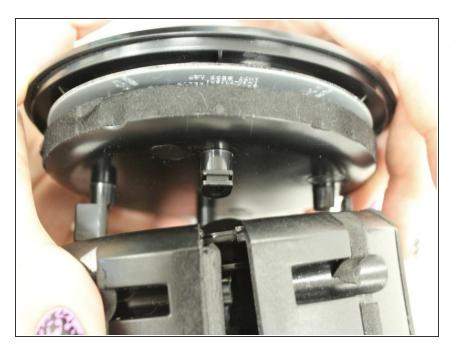
Separate the control panel from the base.
