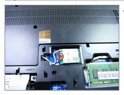
Unscrew the 3mm Phillips #1 screw that holds the WLAN card in place.
