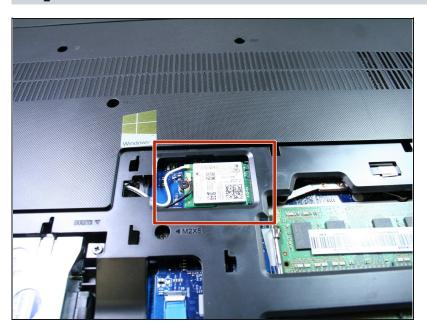
The wireless LAN card is located at the center of the laptop.
