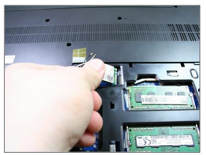
• Gently remove the WLAN card out of its slot.
