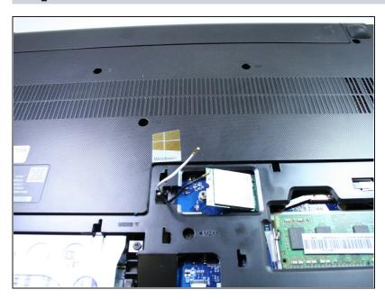
• Disconnect the black and white cables from the WLAN card.
