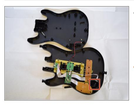
These are the whammy bar components, we highly recommend removing these components before working on other areas of the body as the whammy bar protrudes making it difficult to rest on a flat surface.
