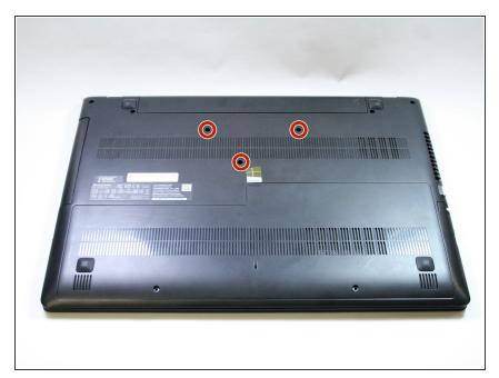
Unscrew the three 6mm Phillips #1 screws from the upper back cover.
