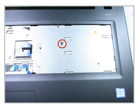
Remove the 6mm Phillips #1 screw that sits in the center of the front plate below the keyboard. This screw sits between two adjacent tabbed holes.
