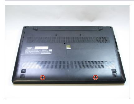
Unscrew the two 7mm Phillips #1 screws that hold the bottom back plate in its place.
