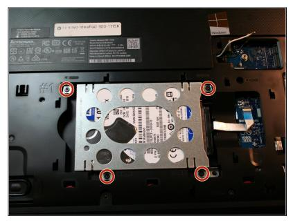
• Unscrew the four 6mm Phillips #1 screws that hold the hard drive frame in place.
