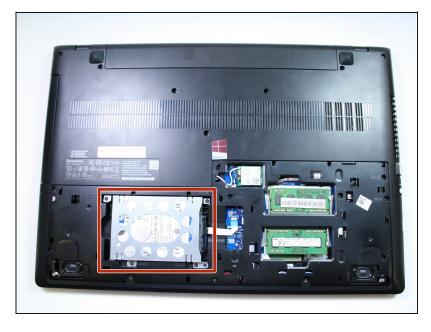
The hard drive is located at the bottom of the laptop.
