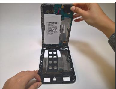
Holding the bottom of the device, lift the front panel from the back panel.
