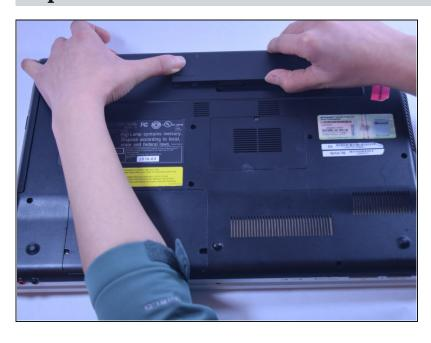
While holding the release slide, use your thumb to lift the lip of the battery to pull it out.
