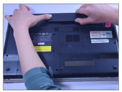
While holding the release slide, use your thumb to lift the lip of the battery to pull it out.
