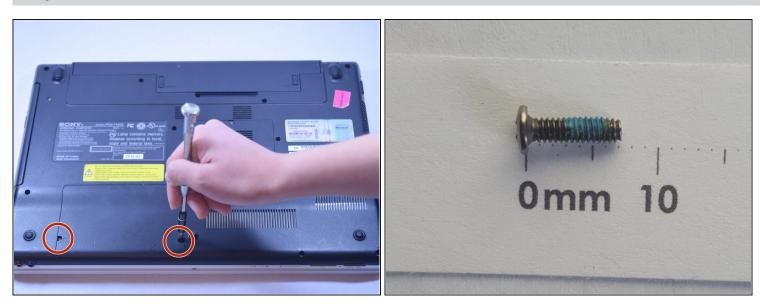
• Using the Phillips #01 Screwdriver, remove the two 7mm screws.
