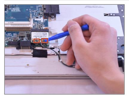
• Carefully remove the antenna plugs.
