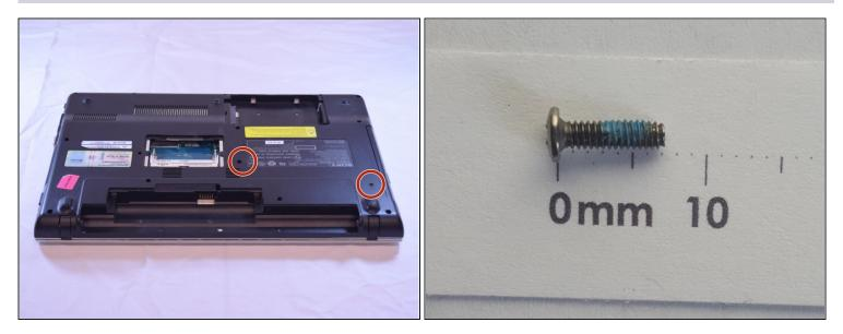
• Remove the 7mm screws with the Phillips #1 Screwdriver.
