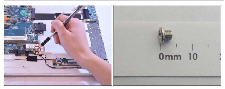
• Remove the 3mm screw with the Phillips #01 Screwdriver
