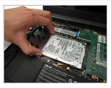
Slide the hard drive in the direction away from the connector and lift it up to remove it.
