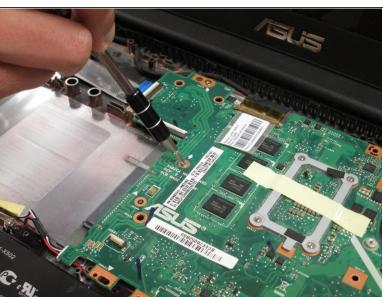
Remove the four 5.5mm screws using the Phillips #0 screwdriver.
