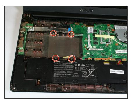
Remove the four 5mm screws from the hard drive mounting bracket using the Phillips #0 screwdriver.
