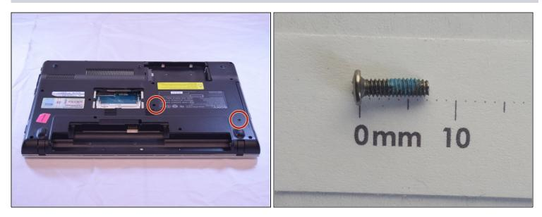
• Remove the 7mm screws with the Phillips #1 Screwdriver.
