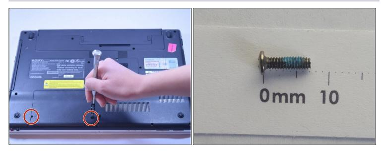
• Using the Phillips #01 Screwdriver, remove the two 7mm screws.
