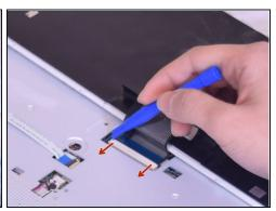
$\triangle$  Carefully pull the keyboard back to expose ribbon connector.
