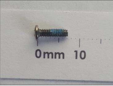
• Remove the 7mm screws with the Phillips #1 Screwdriver.
