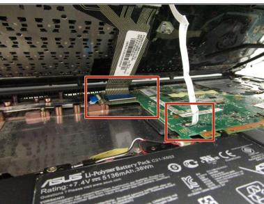
Partially lift the panel up, revealing the two cables connected to the motherboard.
