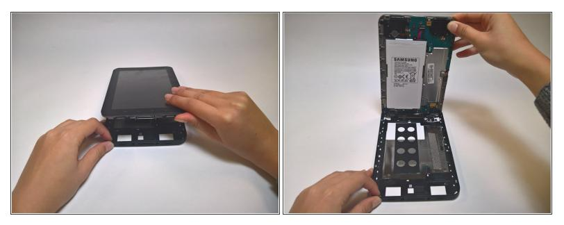
• Holding the bottom of the device, lift the front panel from the back panel.
