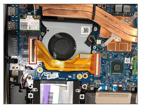
• One of the fans will have a connector that partially covers it. Pull the connector loose by flipping up the plastic clamps on both ends and follow steps 2-4.
