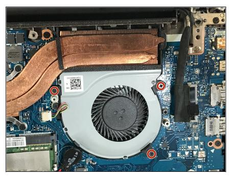
Unscrew and remove the four 5mm Phillips #0 screws from the cooling fan.
