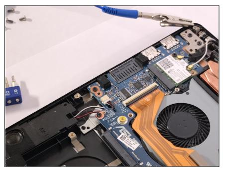
Attach an <u>anti static wrist strap</u> to your hand and clip to the laptop case.
