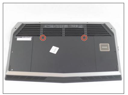
Unscrew and remove the two 4mm Phillips screws from cover.
