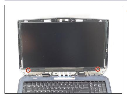
Unscrew and remove the two 2mm Phillips screws from the bottom of the display.
