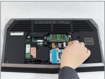
• Unplug the black wire with the yellow tag to disconnect the battery.
