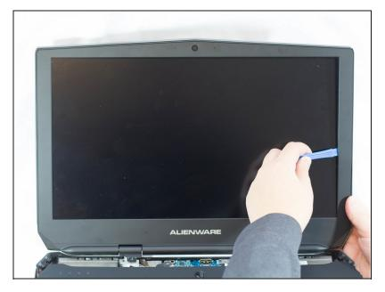
Using the plastic opening tool, pull display casing away from main body.
