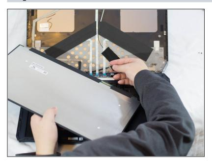
Disconnect plugs connecting the display to the main body.
