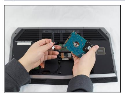
• Remove the plug from the Hard Drive.
