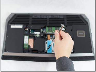
• Unscrew and remove the four 3mm Phillips #1 screws holding the hard drive in place.
