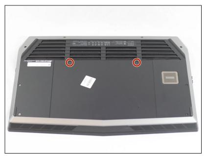
Unscrew and remove the two 4mm Phillips #1 screws from the cover.
