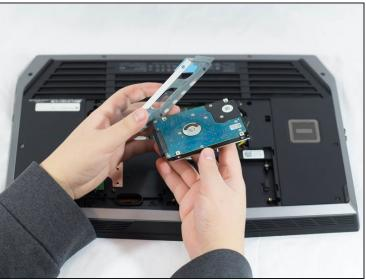
• Unscrew and remove the four 2mm Phillips #1 screws holding the casing together.
