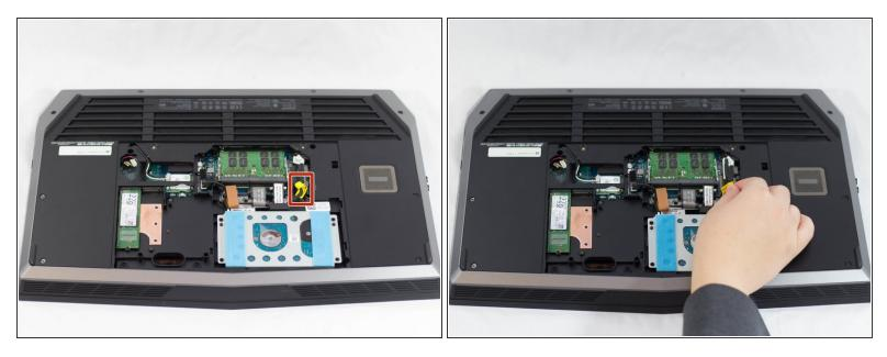
• Unplug the black wire with the yellow tag to disconnect the battery from the RAM stick.
