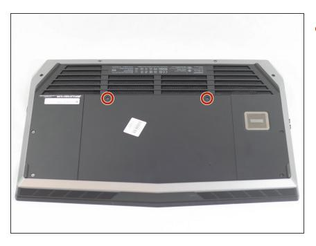
Unscrew and remove the two 4mm
