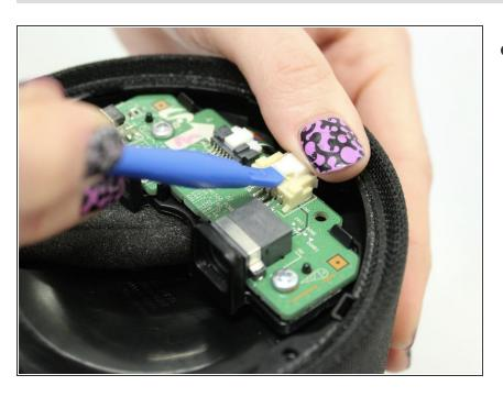
While stabilizing the Port Panel remove the two ribbon cables one at a time by pressing the locking clip down on the ribbon cable connectors and pulling the connector away from the Port Panel.
