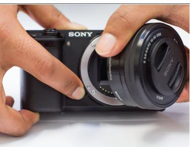
Use the finger, press and hold the release black circle button (on the bottom) next to the lens on the front of the camera. Twist the lens counterclockwise and pull it off.
