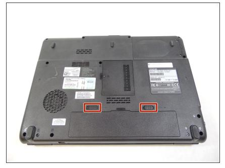
Slide the lock tabs outward. The right tab will lock into place, but the left tab must be held in place.
