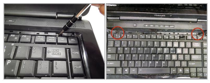
Remove the 3.6 mm Phillips head PH000 screws securing the keyboard.
