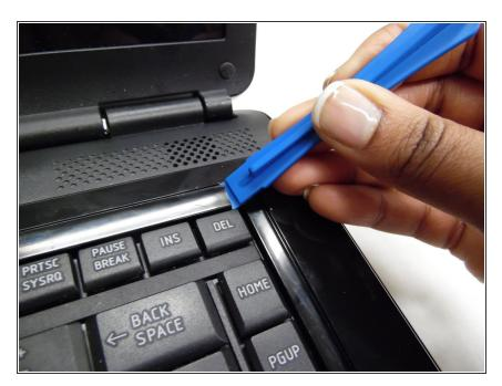
Use a plastic opening tool to lift out keyboard lining portion located at the top of the keyboard.
