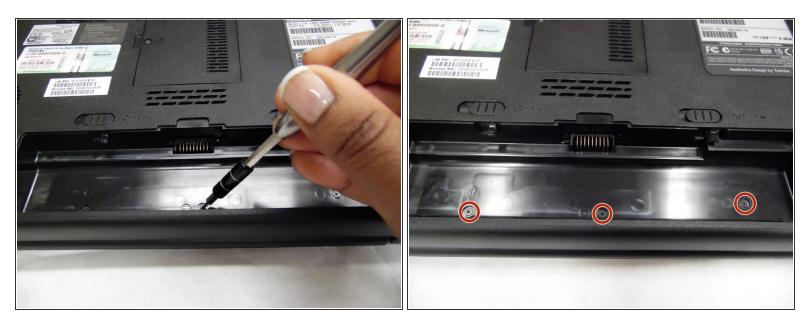
Once the battery is removed, locate and unscrew the 3.2 mm PH1000 Phillips head screws that are underneath the battery.
