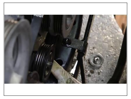
• <u>On the bottom</u> of the idler pulley, loosen the 12mm bolt .
