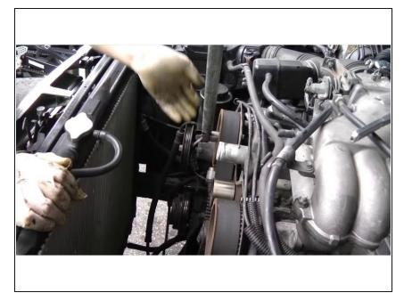
• <u>Line up the</u> camshafts by rotating the big pulley until the notches line up .
