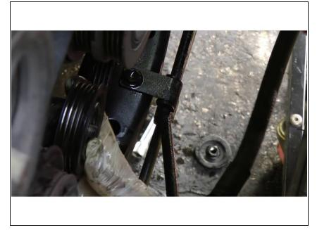
• <u>Remove the 12mm</u> bolt with a washer from the idler pulley .
