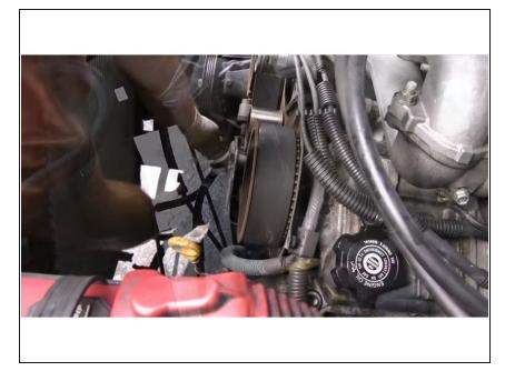
• <u>Loosen the bolts</u> holding the water pump and remove the water pump.
