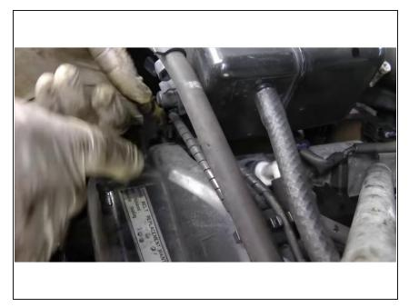
• <u>Take off the</u> spark plug wires .
