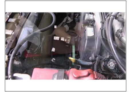
• <u>Loosen up the</u> idler pulley by getting underneath the car and removing the 12mm bolt at the bottom of the idler pulley.
