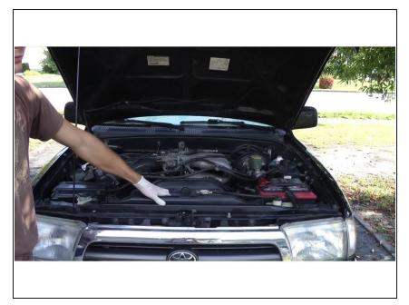
• <u>Begin by removing</u> the fan cover which has four 10mm bolts .
