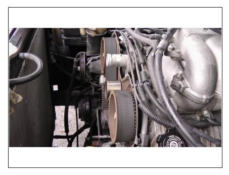
• <u>Line up the</u> notches on the camshafts to set the timing before removing the belt .
