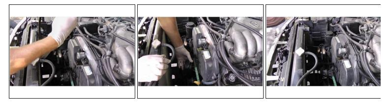
• <u>Remove the pulleys</u> with the four 8mm bolts.
