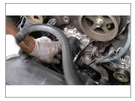
• <u>Remove the old</u> water pump and thermostat housing .
