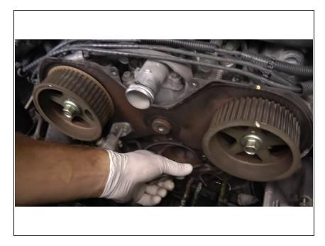
• <u>Scrape off the</u> old gasket from the water pump housing and block .
