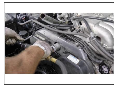
• <u>Remove the ten</u> 10mm bolts on the timing cover .
