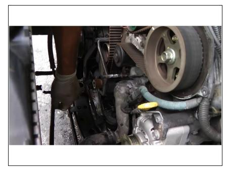
• <u>Remove the bottom</u> cover by taking off the two 10mm bolts .
