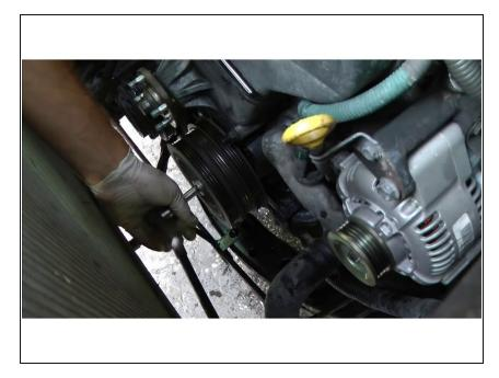
• <u>Remove the nut</u> that holds the pulley in place, which should be torqued down to 250 lbs .
