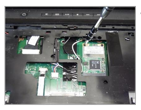
Unscrew both 3 mm Phillips head PH1 screws and allow the wireless card to pop up.
