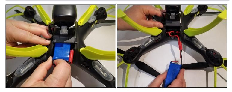
• Carefully pull out battery, pulling out wires first.
