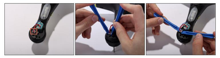
• Unclip the motor cable from the shells housing using two pry tools. Repeat the same procedure for the other three arms.
