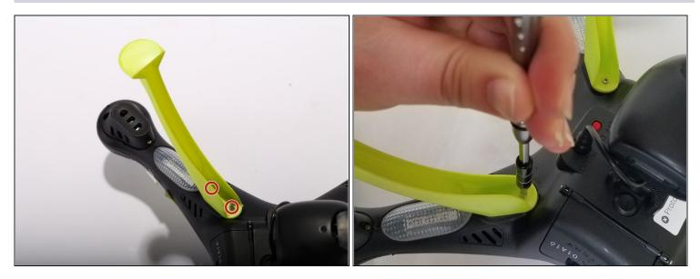
• Unscrew two 9 mm screws located inside the legs. Repeat the same procedure for the other three legs
